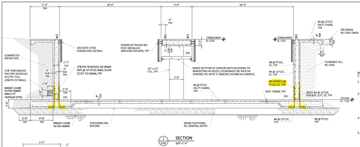
The lap splice length is specified in Note 14 of the Concrete section in Sheet S-01. As shown in Sheet S-04, the bottom of the dowels is at the bottom of the grade beam with 3" of concrete cover.
