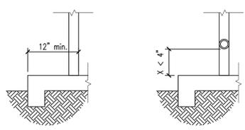
Figure 405.9.1 Extended Floor or Ground Surface Edge Protection
