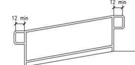
Figure 505.10.1 Top and Bottom Handrail Extension at Ramps
