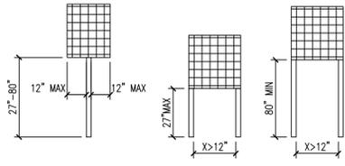
Figure 307.3 Post-Mounted Protruding Objects
