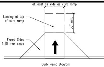
Figure 406.6 Diagonal Curb Ramps
