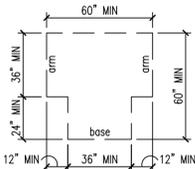
Figure 304.3.2 T-Shaped Turning Space
