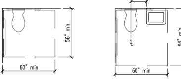
Figure 604.3.1 Size of Clearance at Water Closets Figure 604.3.2 (Exception) Overlap of Water Closet Clearance in Residential Dwelling Units
