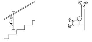
Figure 505.4 Handrail Height Handrail Clearances
