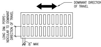
Figure 302.3 Elongated Openings in Floor or Ground Surfaces
