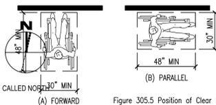
Figure 305.5 Position of Clear Floor or Ground Space
