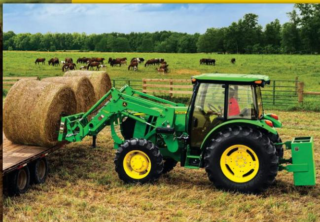
With 9F/3R SyncShuttle and 12F/12R PowrReverser available on 55-75 horsepower models and a 12F/12R PowrReverser and 24F/12R PowrReverser transmission available on 85 and 100 horsepower models you'll have easy directional control (forward and reverse) and speed-matching for any application.
