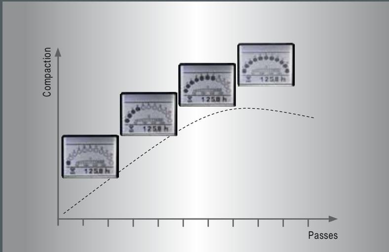
ECONOMIZER knows when full compaction is reached: The lighting strip shows the degree of compaction and warns of over-compaction.
