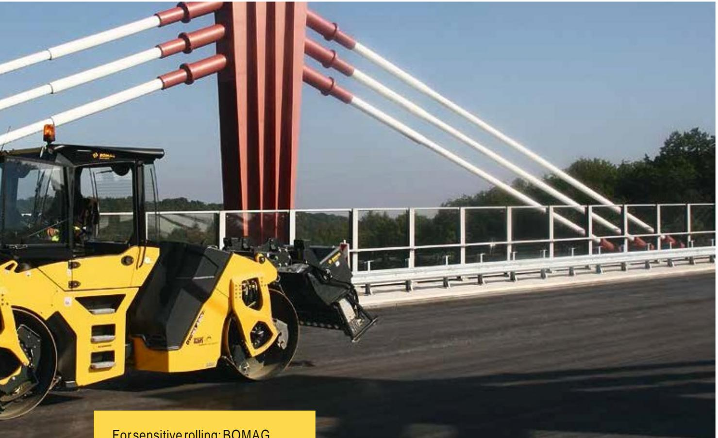
For sensitive rolling: BOMAG tandem rollers with TanGO oscillation. Careful compaction on seams & bridges.
