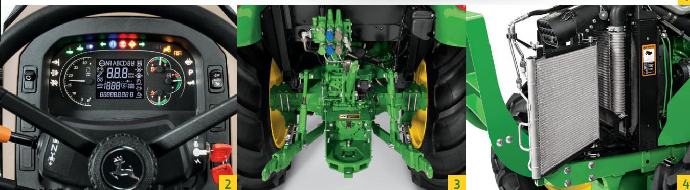
1. New sloping hood on 5E 4 cylinder. 2. New LCD instrument cluster. 3. New standard sway bars and telescoping draft links. 4. New slide out condenser, radiator screen, tilt-able charge air cooler, and slide out condenser on 4 cylinder cab models.
