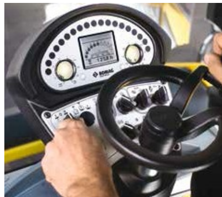
The driver always has all the essential displays safely in view. Operating the switches is simple and quickly becomes second nature.
