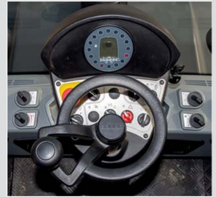
Cockpit design places controls within easy reach and provides unobstructed visibility
